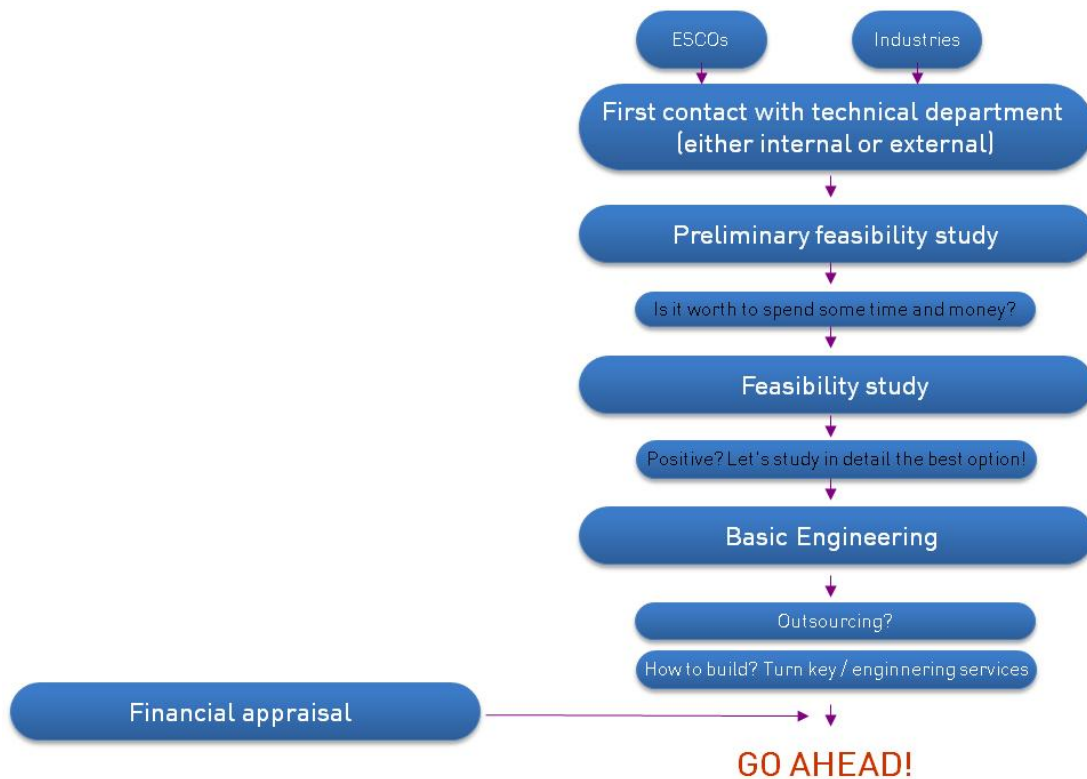
Figure 1: Flowchart detailing the steps an industrial polygeneration project goes through before being given the go-ahead by a company.
